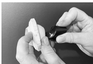
Restricting a Ring and Ball fitting
