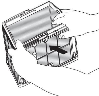
**6.2.2** Dismantle the panels, starting by pressing on panel 1 using your thumbs.
